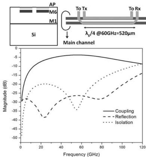
Fig. 2. On-chip directional coupler and its simulated performance
