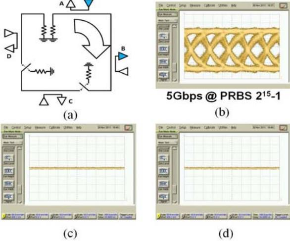
Fig. 9. Eye diagrams when drop A transmits and only B receives
