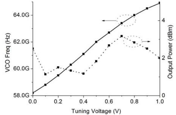
Fig. 6. Transmitter output frequency and calibrated output power
