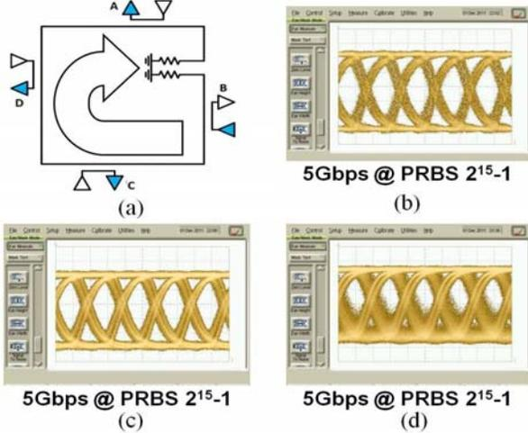
Fig. 8. Eye diagrams when drop B multi-casts to drops C, D, A
