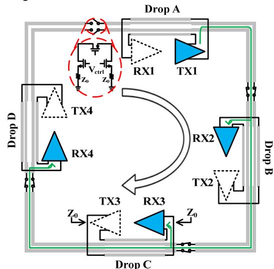
Fig. 1. 4-drop RF-I with Arbitration Capability (Drop A multicasts)
