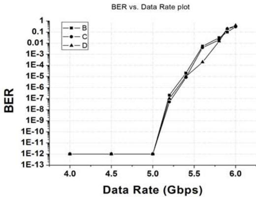
Fig. 10. Measured BER vs. data rate at different drops
