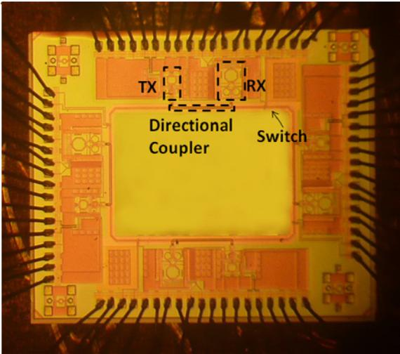
Fig. 5. 5Gbps RF-I with multi-drop and arbitration die-photo
