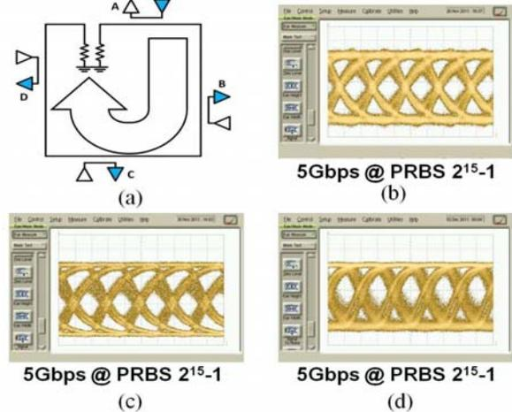
Fig. 7. Eye diagrams when drop A multi-casts to drops B, C, D
