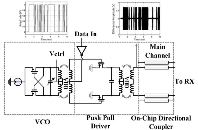
Fig. 3. 60GHz ASK transmitter
