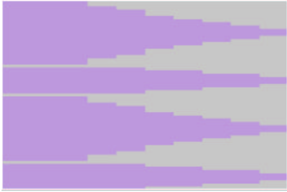
Figure 5. The OWS sizing result for a 4-bit bus with 3 \times pitch between adjacent lines.
