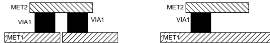
Figure 5. Via spacing violations in a two layer routing problem can be easily corrected because Property 3 implies that there cannot be any obstacles between the two vias. Therefore, the vias (either one or both depending on other connections to the vias) can be replaced with a wire segment at the metal layer.
