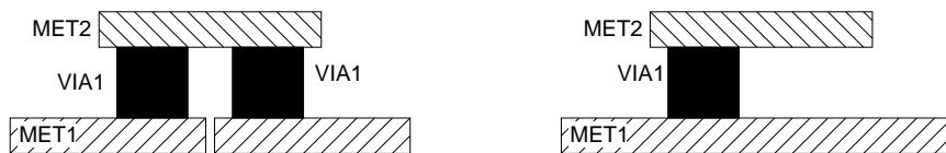
Fig. 5. Via spacing violations in a two layer routing problem can be easily corrected because Property 3 implies that there cannot be any obstacles between the two vias. Therefore, the vias (either one or both depending on other connections to the vias) can be replaced with a wire segment at the metal layer.
