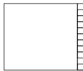
Fig. 6. Block aspect ratios may all remain small, even when some subregion has a large aspect ratio.
