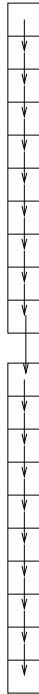
Figure 6: An example of the artificial path on an Altera Stratix device. The path traverses all the LEs of a LAB before moving to an adjacent LAB.
