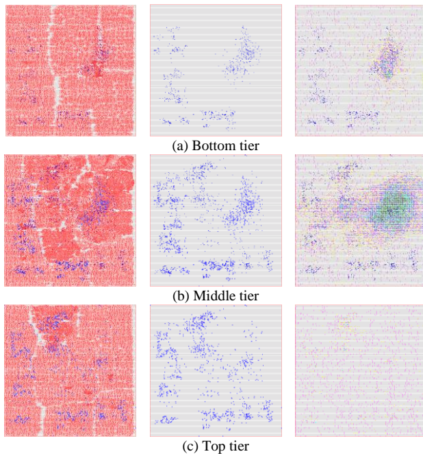
Fig. 5. The 3D placement by mPL-3D, the TS via distribution, and the routing congestion analysis by Cadence Encounter
