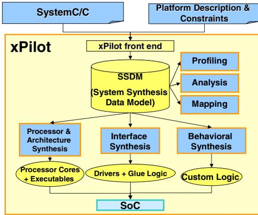
Fig. 1. xPilot system-level synthesis framework.
