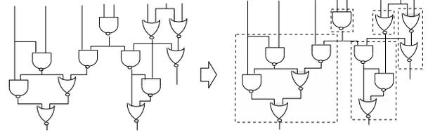
Figure 3 MFFC decomposition of the network in Figure 2
