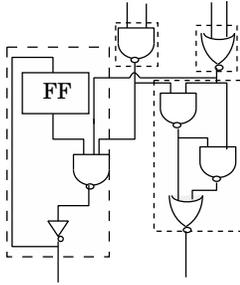
Figure 4 MFFC decomposition of a sequential circuit
