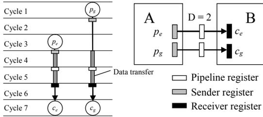
Figure 5. Simultaneous transfers using two data links.
