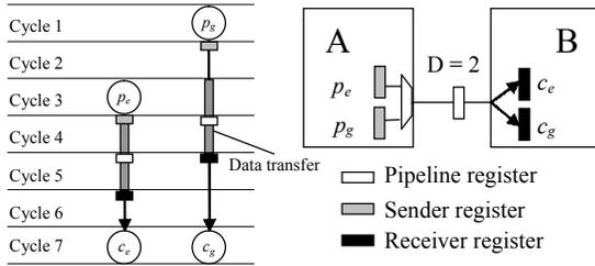
Figure 6. Scheduled transfers using only one data link.
