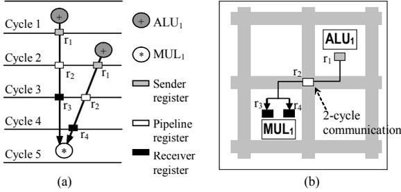
**Figure 3. Illustration of the interconnect pipelining and sharing in RDR-Pipe**
